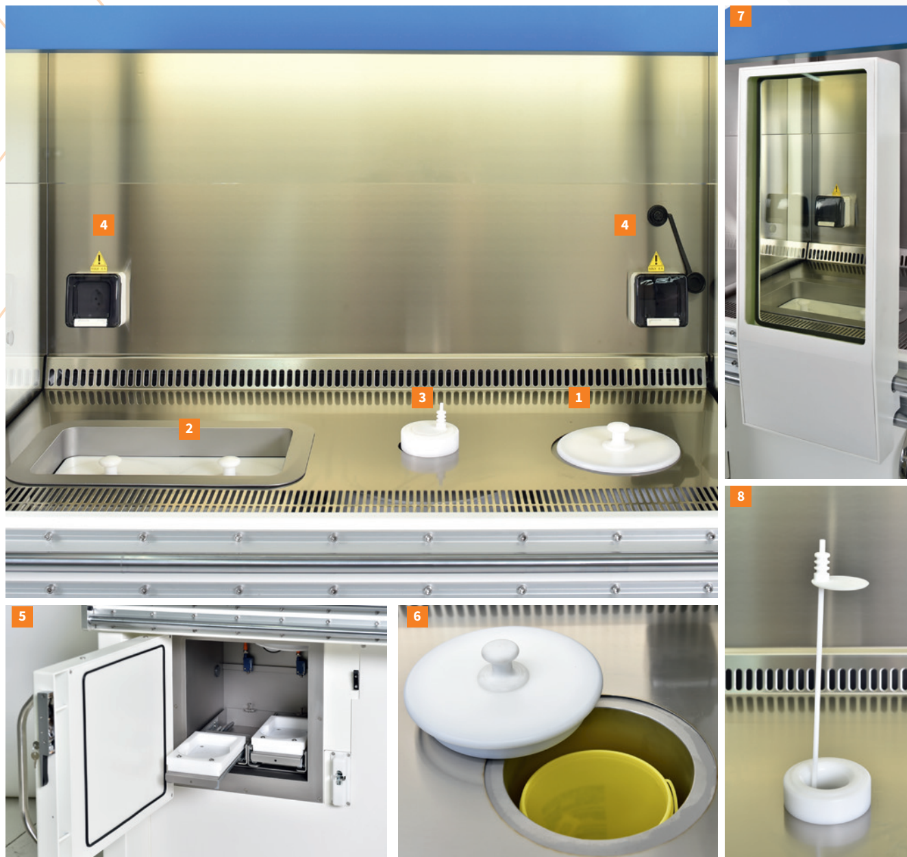
1 | 1 waste bin 2 | 2 independent accesses for each generator 3 | 1 access for the dose calibrator 4 | 2 socket emplacements (electrical, USB, RJ45) 5 | 1 shielded lockable compartment for 2 generators, equipped with 2 loading trays and 2 independent lifts 6 | Access to the waste compartment 7 | Sliding, removable and retractable lead glass screen 8 | Posilift system (raising and lowering of the dose calibrator dipper by foot control)
